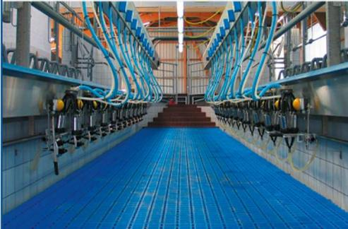
The temperature neutral panels TRAPPER and STEPPER ensure a safe and ergonomically designed workplace.
